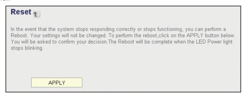
Apply — Click to reset the router. It will be operational again after a few minutes. **NOTE:** This function does not change any settings you have made. It simply restarts (reboots) the router — just as Start / Shut Down / Restart reboots your computer — freeing up memory and system resources for more stable operation.
