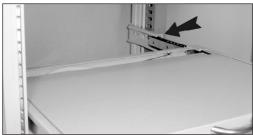
4. Fasten the console drawer to the outside of the front vertical uprights using the four screws provided. The metal brackets (as indicated by the far arrow) support the rear side of the console.
