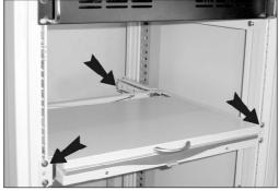
Remove both rear brackets and slide the drawer halfway out to balance its weight. (The front brackets hold the drawer.) NOTE: The image at right is a rear (KVM switch module-side) view.
