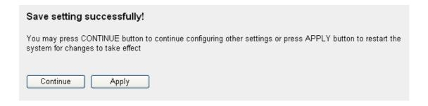
Click "Continue" to go back and continue with the router setup procedure, or click "Apply" to reboot the router so the settings will take effect. (Wait for about 30 seconds while the router is rebooting.)
