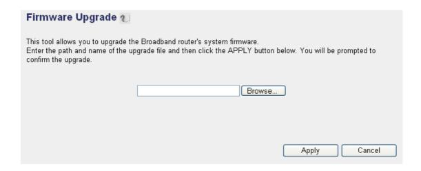
Click "Browse" first and you'll be prompted to provide the filename of the firmware upgrade file. Download the latest firmware file from www.intellinet-network.com and use it to upgrade your router. After a firmware upgrade file is selected, click "Apply" and the router will start the firmware upgrade procedure automatically. The procedure may take several minutes.
