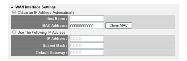
Select how you obtain an IP address from your service provider. You can choose "Obtain an IP address automatically" (equal to DHCP — refer to "Cable Modem" above), or "Use the following IP address" (i.e., a static IP address).
