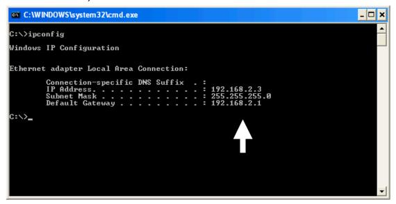
NOTE: If the IP address of the default gateway is not displayed, or if the address following "IP Address" begins with "169," re-check the network connection between your computer and router, and/or go to the beginning of this chapter to re-check each step of the network setup procedure.
