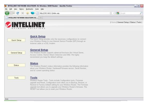
NOTE: If you can't see the Web management interface and you're being prompted to input the user name and password again, it means you didn't input the user name and password correctly: Re-enter the user name and password. If you're certain the user name and password you entered are correct, refer to 4-2 Troubleshooting to perform a factory reset to set the password back to its default value.
