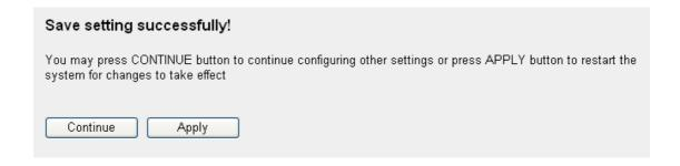
Click "Continue" to go back and continue with the router setup, or click "Apply" to reboot the router so the settings will take effect. (Wait for about 30 seconds while router is rebooting.)
