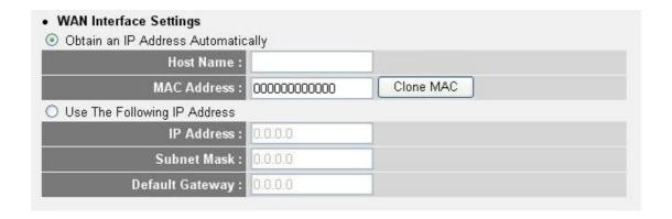
Select how you obtain an IP address from your service provider here. You can choose "Obtain an IP address Automatically" (equal to DHCP; refer to the Cable Modem section above), or "Use the Following IP Address" (i.e., static IP address).
