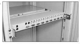
Slide the console drawer out to gain access to the connecting screws. Push the KVM switch module evenly toward the connector attached to the console drawer and lock both units together by tightening the screws indicated by the arrows.
