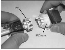
3. Connect the cap with the IDC base, using the guidepost for proper alignment.
