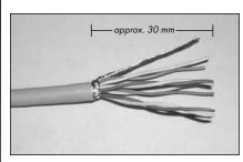
1. Strip away approx. 30 mm of the cable jacket. Separate the wires into four pairs while isolating the ground wire.
